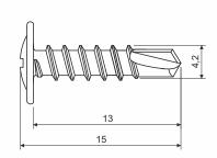
product description: screw designed to connect two metal parts with a sheet thickness of up to 2.0 mm
