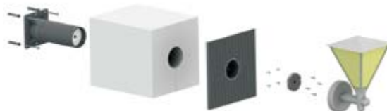
MDZ XL, MDZ XL 300 - mounting desk into thermal insulation
