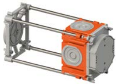
length of spacer bars = thickness of the wall to be built - 45 mm
